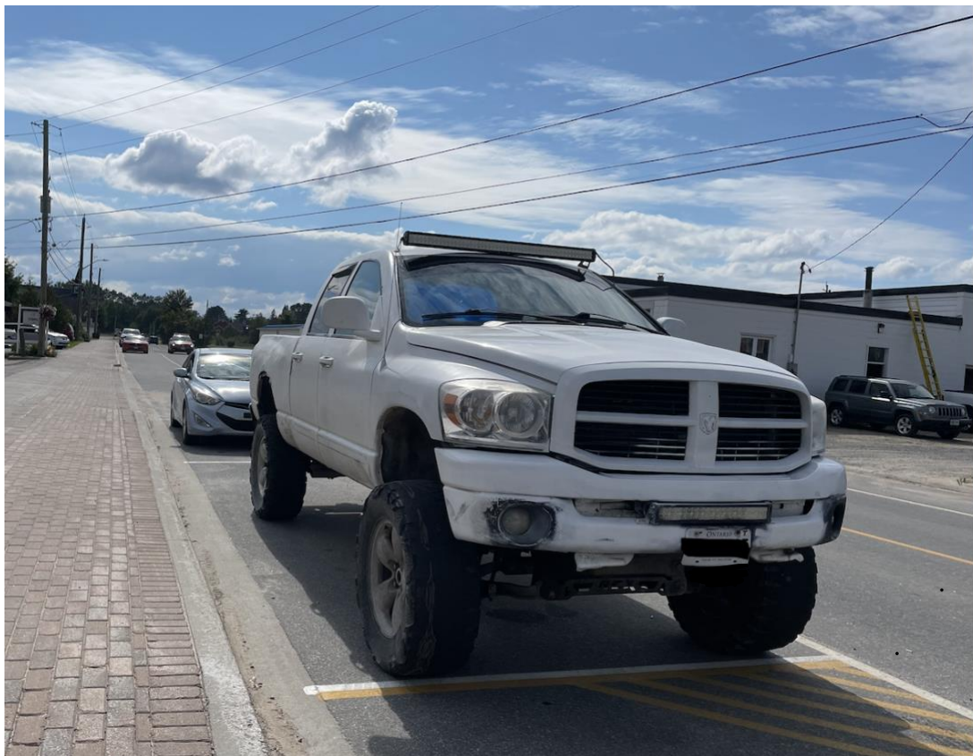
Image 2: Pickups have grown dramatically in size, while specific design features such as blunt, high front ends increase the likelihood of more severe injuries to vulnerable road users in crashes. Vehicle modifications, as in this photo, may exacerbate the risks of design features. A concern for the safety of road users outside of these vehicles is yet to be apparent in government safety standards and policies. (Photos by Albert Koehl, unless otherwise noted)
