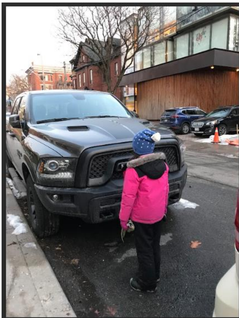
Image 3: Research studies show that in crashes with pedestrians, light trucks are particularly deadly to children. Reducing the height of a vehicle's front-end to below 1.25 metres would save many lives. (Photo: Adriana Bravo)
